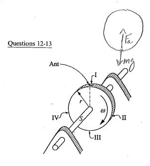
An ant of mass m clings to the rim of a flywheel of radius r, as shown above. The flywheel rotates clockwise on a horizontal shaft S with constant angular velocity  $\omega$ . As the wheel rotates, the ant revolves past the stationary points I, II, III, and IV. The ant can adhere to the wheel with a force much greater than its own weight.
