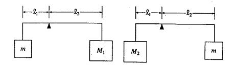
35. A rod of negligible mass is pivoted at a point that is off-center, so that length  $\ell_1$  is different from length  $\ell_2$ . The figures above show two cases in which masses are suspended from the ends of the rod. In each case the unknown mass m is balanced by a known mass,  $M_1$  or  $M_2$ , so that the rod remains horizontal. What is the value of m in terms of the known masses?
