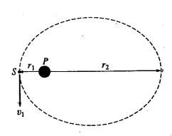
32. A satellite S is in an elliptical orbit around a planet P. as shown above, with  $r_1$  and  $r_2$  being its closest and farthest distances, respectively, from the center of the planet. If the satellite has a speed  $v_1$  at its closest distance, what is its speed at its farthest distance? IW = IW
